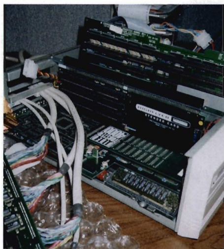
The insides of the A4000. Tread carefully as there are many critical components here. Note too that it is not necessary to totally unhook the Flyer board and its hookups. It's also a good idea to keep all removed screws, washers and items in a cup for safe keeping. The installation looks scarier than it actually is!
